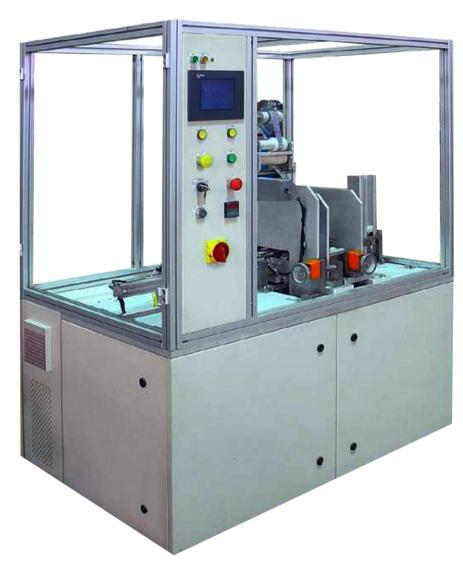
Hot stamping machine for application of hologram and signature panels for ISO pvc plastic cards.
